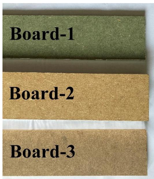
**Figure 1** Uncoated industrial fibreboards used for the thermo-hydrolytic disintegration process.
