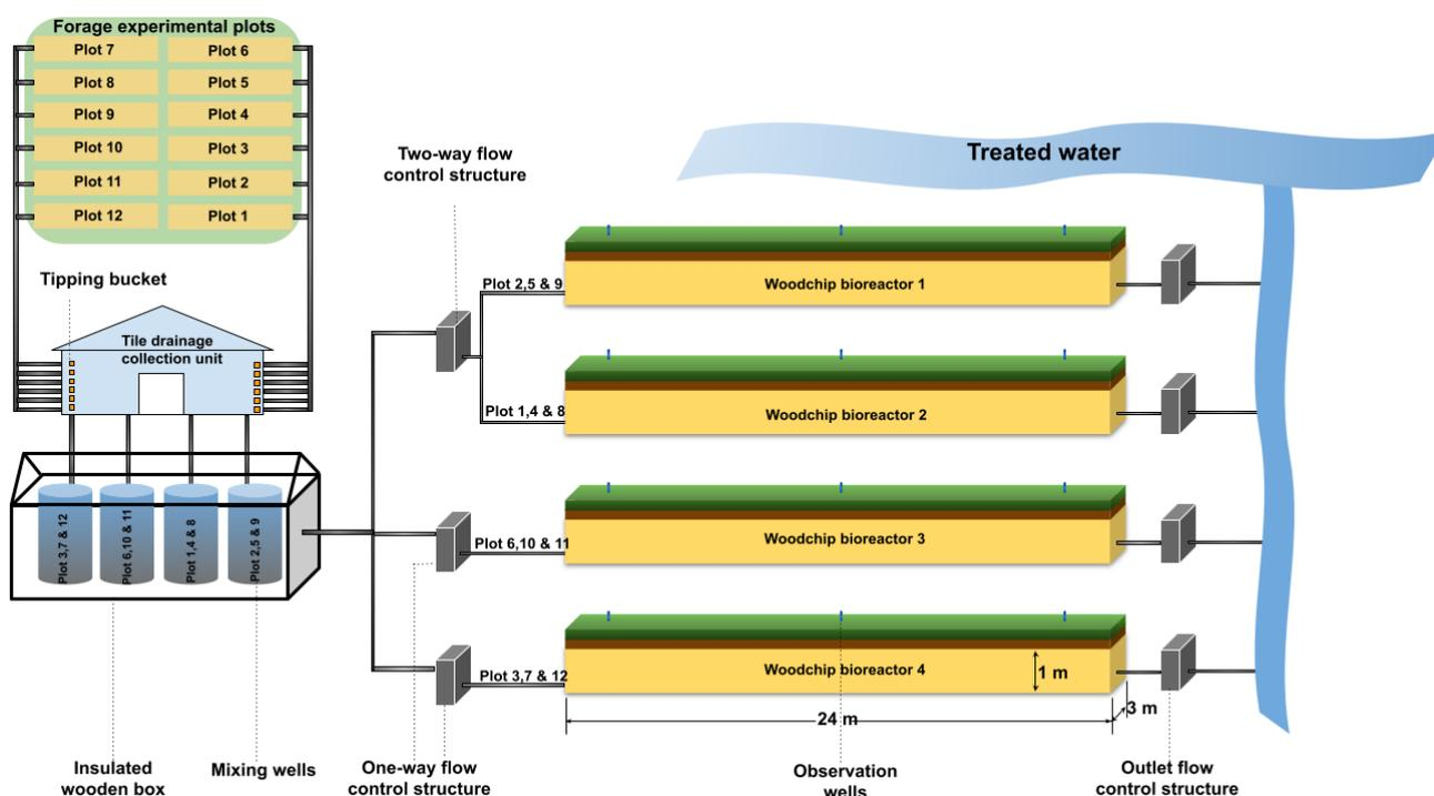
**Figure 1** Novel field scale experimental and woodchip bioreactor design set-up at St. John's Research and Development Centre.
