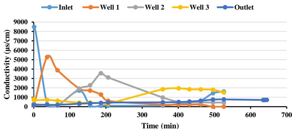
Figure 4 Tracer movement at the bioreactor over the period of time.
