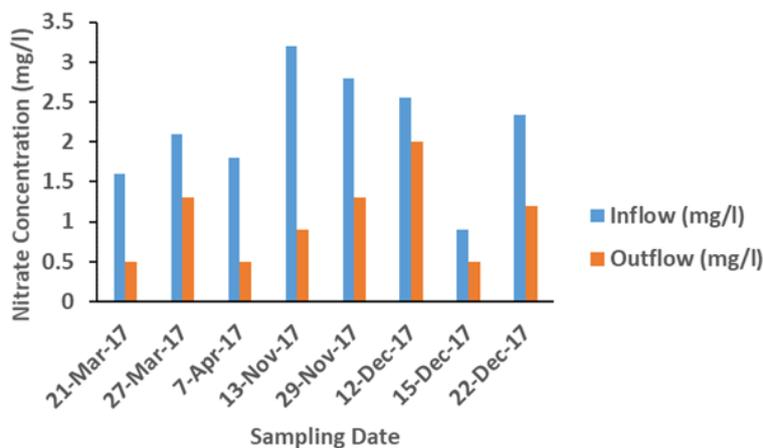
**Figure 7** N inflow and outflow concentration of field scale woodchip bioreactor, St. John's, NL.
