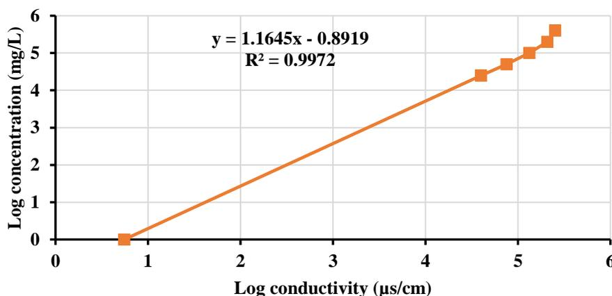
**Figure 3** Calibration curve of log conductivity versus log concentration used to calculate associated parameters.
