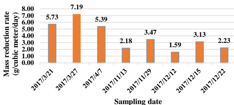
**Figure 8** MRR of N removal at bioreactor (#1), St. John's, NL.
