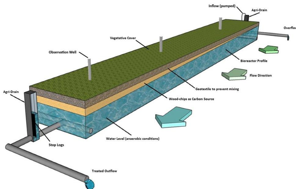
**Figure 2** Schematic diagram of one of the four replicated bioreactors at St. John's Research and Development Centre where tracer testing was performed. Arrows indicate the water flow direction and monitoring wells are illustrated along the flow path.
