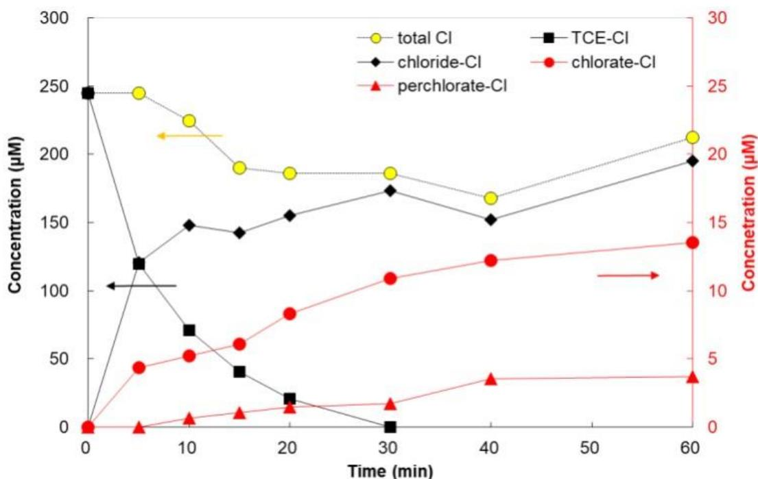
**Figure 5** Formation of inorganic chlorinated byproducts during the degradation of TCE in the EO process with  $\text{Ti}_4\text{O}_7$  anode. Experimental condition: PFOS  $2 \mu\text{M}$  ( $1 \text{ mg/L}$ ), TCE  $76 \mu\text{M}$  ( $10 \text{ mg/L}$ ),  $\text{Na}_2\text{SO}_4$   $100 \text{ mM}$ , reaction volume  $200 \text{ mL}$ , current density  $20 \text{ mA/cm}^2$ .
