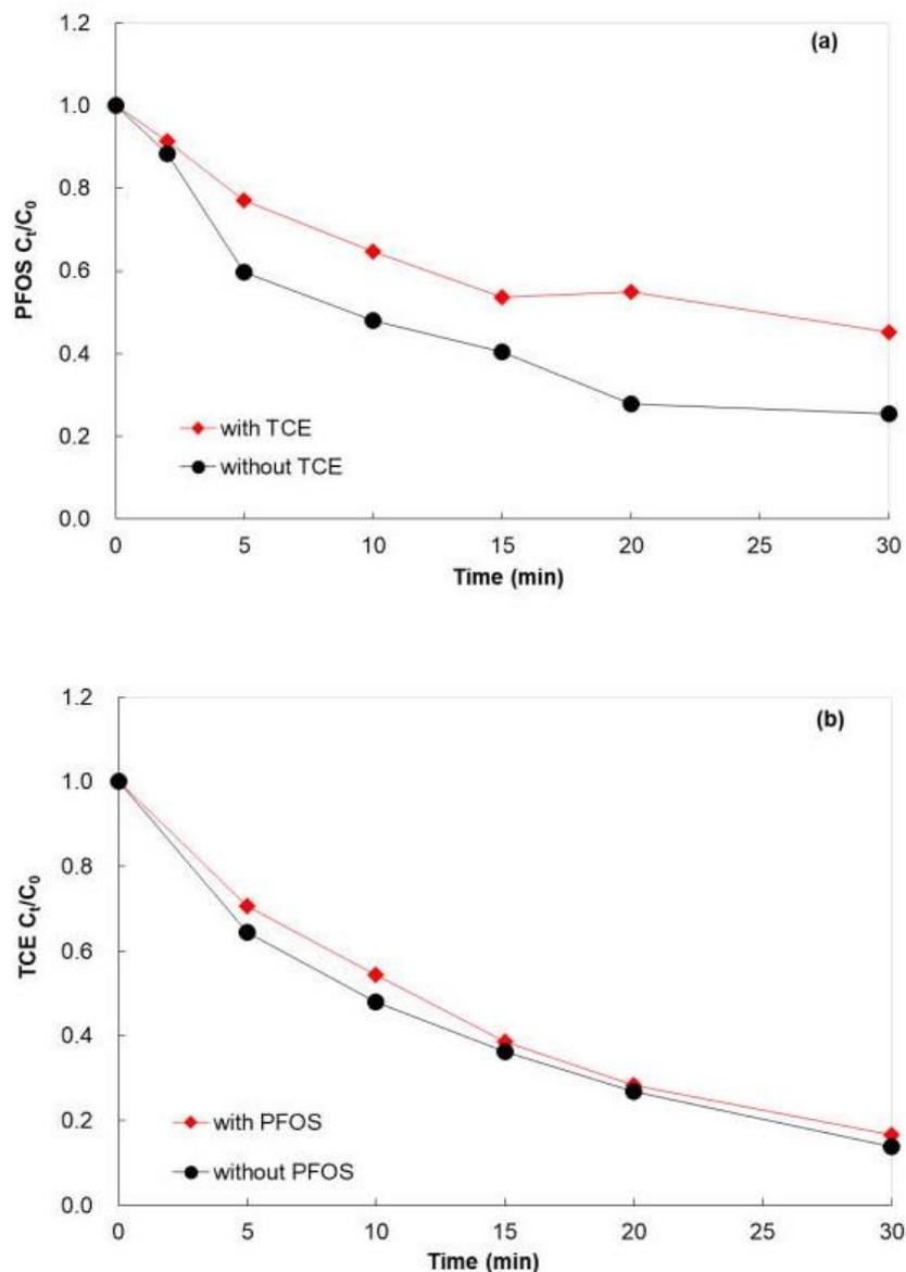
**Figure 2** Removal of (a) PFOS and (b) TCE in the EO process with  $Ti_4O_7$  anode. Experimental condition: PFOS 2  $\mu$ M (1 mg/L), TCE 76  $\mu$ M (10 mg/L),  $Na_2SO_4$  100 mM, reaction volume 200 mL, current density 10 mA/cm<sup>2</sup>.
