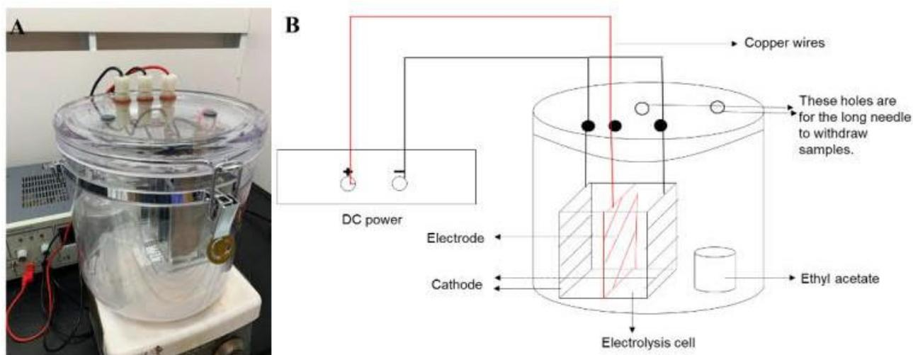
**Figure 1** Picture and scheme of Gas-tight EO reactor.
