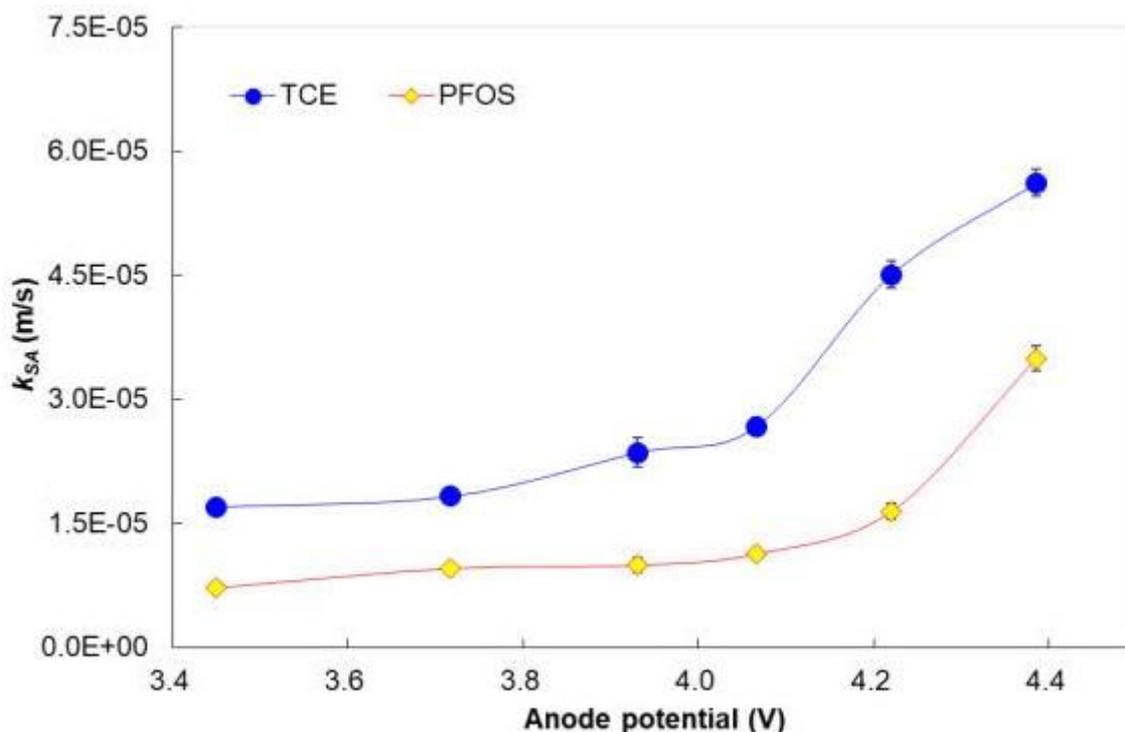
**Figure 3** Relationship of surface area normalized rate constants ( $k_{SA}$ ) of PFOS and TCE and anode potential. Experimental condition: PFOS 2  $\mu$ M (1 mg/L), TCE 76  $\mu$ M (10 mg/L), Na<sub>2</sub>SO<sub>4</sub> 100 mM, reaction volume 200 mL, current density 2.5, 5, 7.5, 10, 15, and 20 mA/cm<sup>2</sup>.
