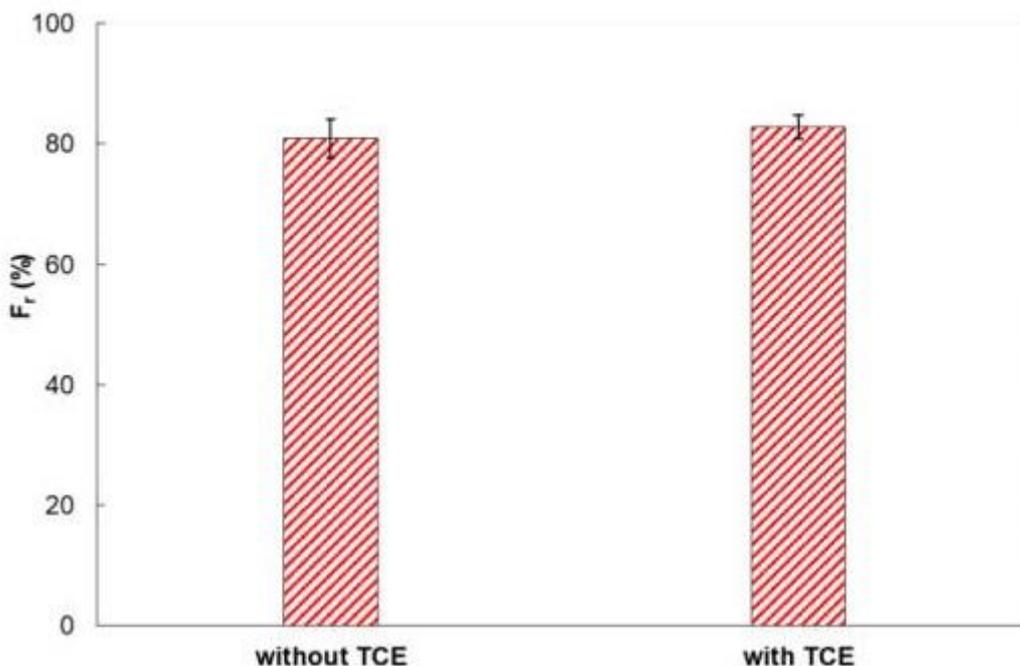
**Figure 4** Fluoride release in the EO process with  $\text{Ti}_4\text{O}_7$  anode. Experimental condition: PFOS  $2 \mu\text{M}$  ( $1 \text{ mg/L}$ ), TCE  $76 \mu\text{M}$  ( $10 \text{ mg/L}$ ),  $\text{Na}_2\text{SO}_4$   $100 \text{ mM}$ , reaction volume  $200 \text{ mL}$ , current density  $10 \text{ mA/cm}^2$ .
