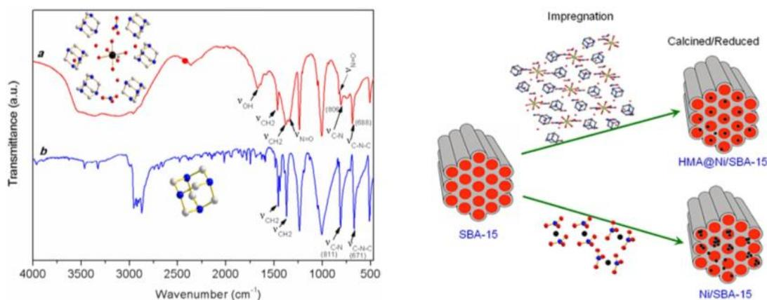
**Figure 2** Left: The FTIR spectra of a: the *as*-synthesized (NO<sub>3</sub>)<sub>2</sub>Ni(H<sub>2</sub>O)<sub>6</sub>(HMA)<sub>2</sub>·4H<sub>2</sub>O complex and b: HMA; Right: The schematic illustration of the improved Ni dispersion for HMA@Ni/SBA-15 compared to Ni/SBA-15 [40].
