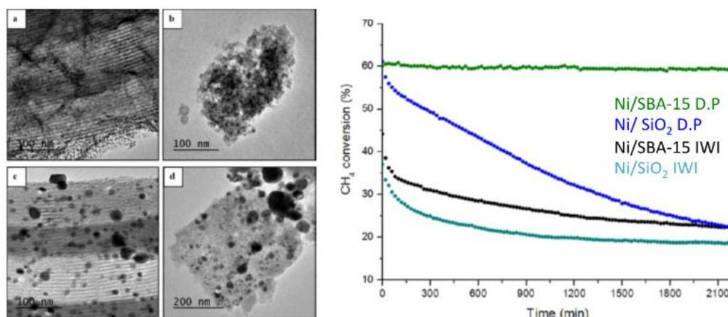
**Figure 3** Left - TEM images of reduced: a: Ni/SBA-15 DP, b: Ni/SiO<sub>2</sub> DP, c: Ni/SBA-15 IWI, and d: Ni/SiO<sub>2</sub> IWI; Right - CH<sub>4</sub> conversion in the reaction of DRM at 750 °C under one of the best GHSV (240 L g<sup>-1</sup> h<sup>-1</sup>) reported [46].
