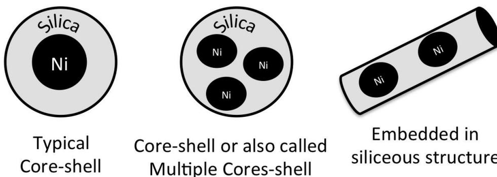
**Figure 4** Different approaches leading to the physical protection of nickel by porous silica.
