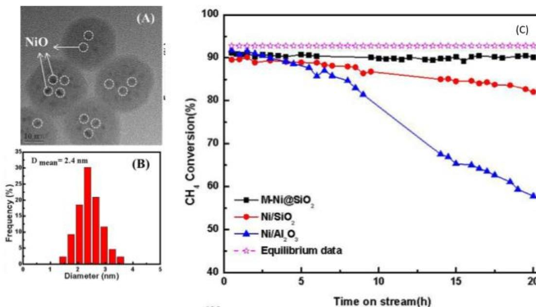
**Figure 5** A and B: TEM and Ni particle size distribution of M-Ni@SiO<sub>2</sub> and C: comparison of the stability of different Ni-based silica or alumina catalysts toward the CH<sub>4</sub> conversion [118].
