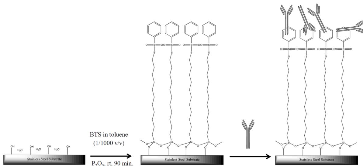
**Figure 1** Schematic showing 'bare' stainless steel substrate (left) coated with BTS linker (centre) and antibodies (right).
