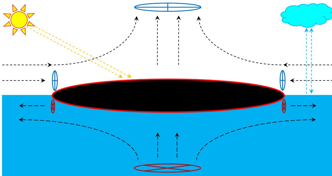
**Figure 5** A model of a floating fuelless electric complex combining solar (black filled oval), wind (blue ovals with +), convection (ovals with horizontal elongation above in the air and below in water), water current (red ovals with X), wave (red perimeter of solar PV), and other fuelless generators. Shown are (reciprocating) convective flows in air (white) and water (blue), sunlight (orange dashed), water evaporation and rain (light-blue dashed arrows). See text in section 3.4.
