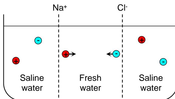
**Figure 4** Electricity from a difference of water salinity is generated using two conductive ion-exchange membranes, one of which is transparent for  $\text{Na}^+$  (but not  $\text{Cl}^-$ ), the other – for  $\text{Cl}^-$  ions.
